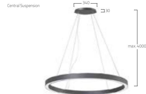
Minimal suspension height for the central suspension
