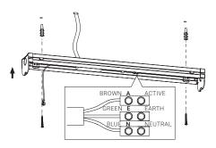
Connect the light source to the base. Press the snap-on button and fix the cover to the base.
